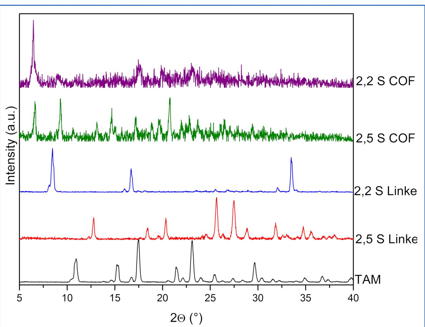
Crystallinity of the samples was confirmed via Powder X-Ray Diffraction. For both materials, two characteristic COF peaks, very comparable to COF 300s hydrated and dehydrated diffraction peaks [2], could be observed around 6.5 and 9° 20. Even after thorough cleaning, a peak belonging to residual TAM could be distinguished in both samples.
