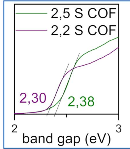
The band gap of the materials was estimated via solid state UV-VIS spectroscopy. As expected, the band gaps of both materials are very comparable and situated in the visible range (quite close to green light). This makes them potentially attractive for use as metal-free photocatalysts.
