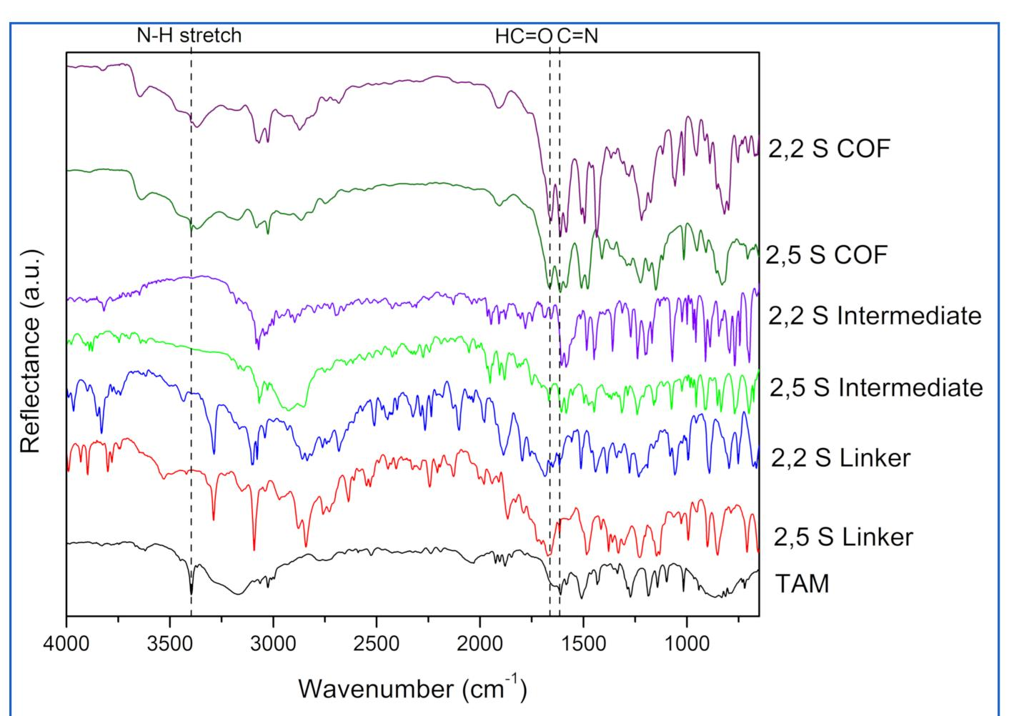
Using FTIR spectroscopy, the formation of COF was confirmed by the appearance of an imine band. However, the partial elimination of starting materials suggested incomplete reaction with remaining aldehyde and amine functions in the COF material.
