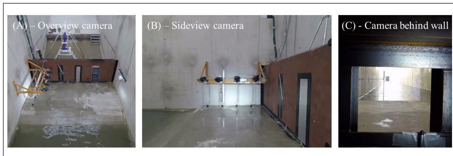
Figure 3.18: Three GoPro 5 Black were deployed during the 'DeltaFlume' experiment. The views from the overview camera (A), the sideview camera (B) and the camera filming through the observation window in the wall (C) were provided.
