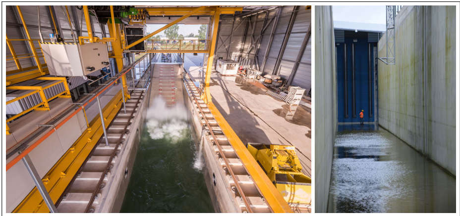
Figure 3.6: Deltares Delta Flume for prototype testing (left figure) and its 9m high blue piston type wave paddle (right figure).
