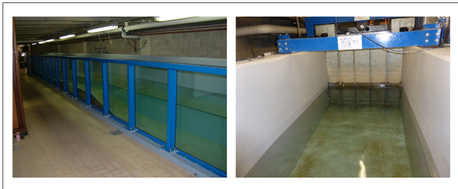
Figure 3.2: Ghent University wave flume facility with glass front along 15m flume width (left figure) and piston type wave paddle (right figure).
