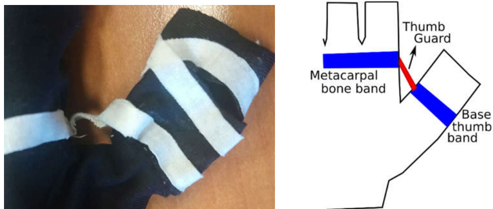
Figure 4. Example prototype for a thumb guard. Two compressive elastic bands (blue) are connected by a non-elastic thumb guard band (red)
