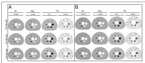
**Fig. 3** Axial slices of the phantom reconstructed using TOF-OSEM for 2, 3, and 4 iterations and 28 subsets for different acquisition times and different isotopes: **a** without PSF and post-smoothing filter and **b** with PSF and 2 mm Gaussian filter
