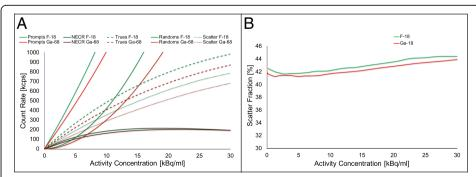
**Fig. 1** NEMA counting rate measurements: count rates (**a**) and scatter fraction (**b**) vs activity concentration for the both isotopes <sup>18</sup>F and <sup>68</sup>Ga. Notice than peak of the NECR curve (**a**) of <sup>68</sup>Ga is lower (at clinical NECR) and appears at higher activity concentrations
