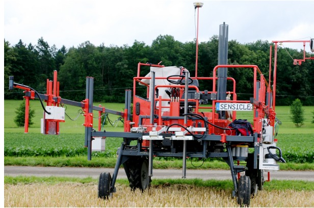
Figure 2. The multi-sensor platform “Sensicle” with the mounted sensors.
