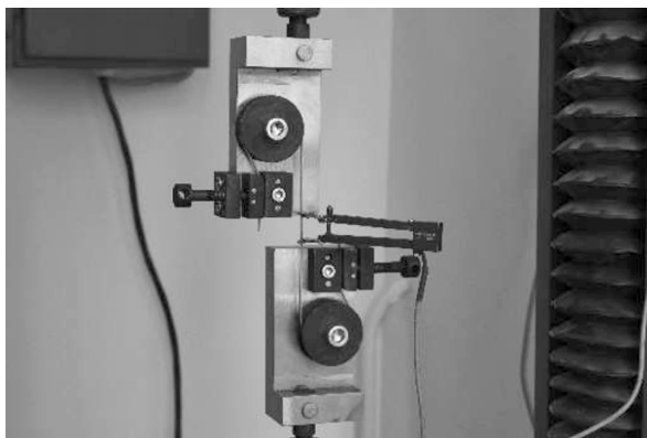
Fig. 1. Grips with a wire and an extensometer aimed at measuring longitudinal deformations installed in a FP-100 machine.
