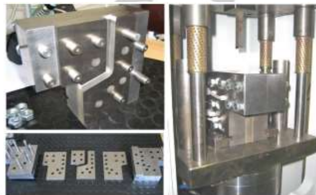
Figure 7. Up and right: the ECAP die used for SPD treatments applied to Mg alloys. The die setting on the press (down) is pushed towards the punch, which pushes the sample for channeling. Up and left: the open channeling die; down-left: tools forming different angle channels ( L_E = 95^\circ, 105^\circ, 115^\circ, 125^\circ and 135^\circ ); right: ECAP system (die and punch)
