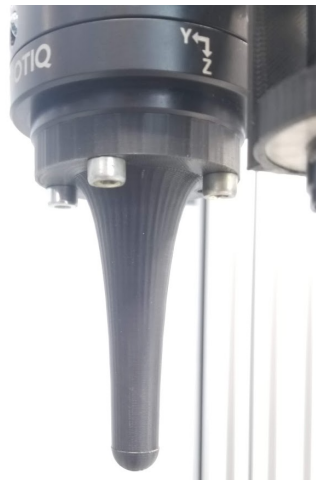
Figure 3.4: FT300 force sensor coupled with the pressing tool
