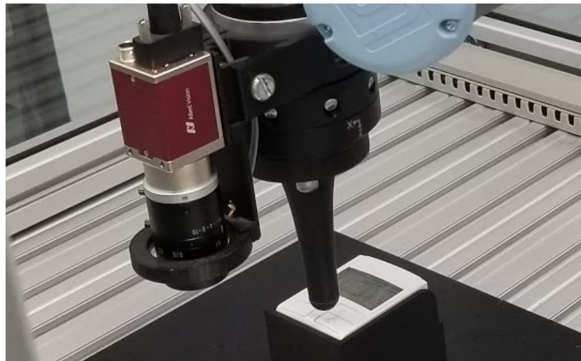
Figure 4.16: Robot pressing the buttons during the inspection task.
