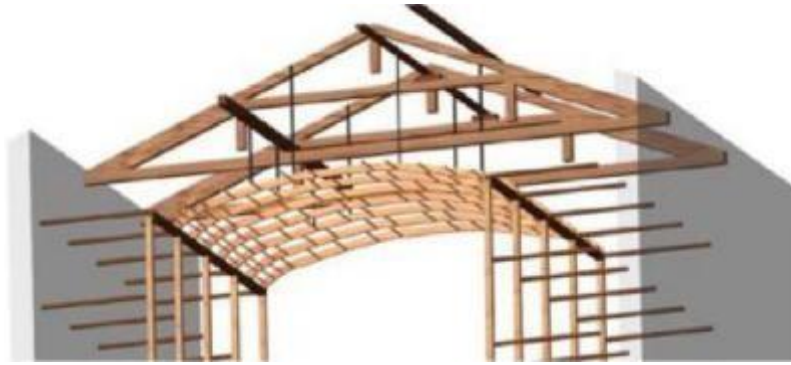
Figure 2. 8 Scheme of the covering reinforcements and the wooden frames of the hall.
