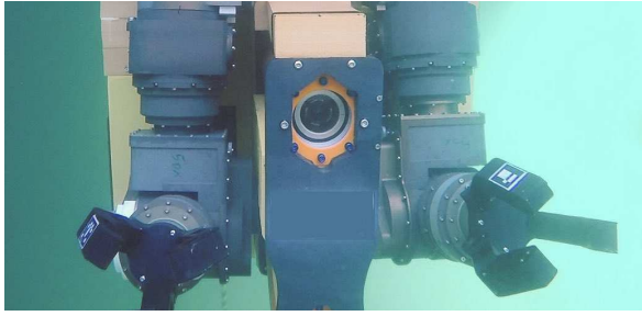
Fig. 1. The DexROV system underwater. In this picture mock up hands have can be recognized.
