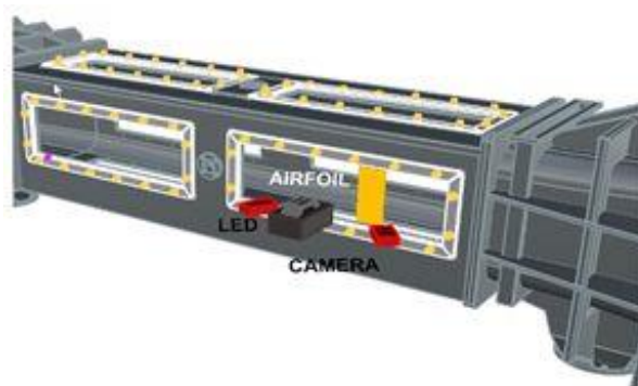
Figure 1: Sketch of the experimental setup at CEIMM (Rome-Italy). The hydrofoil model (orange) is placed in the middle of the tunnel and lighted with LED lamps. Its emission is acquired by a Photron SAX fast camera.
