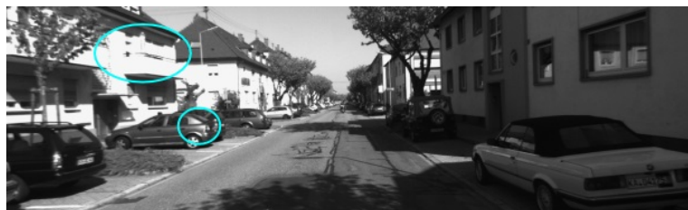
(c) Sensor oversaturation and specular reflections
