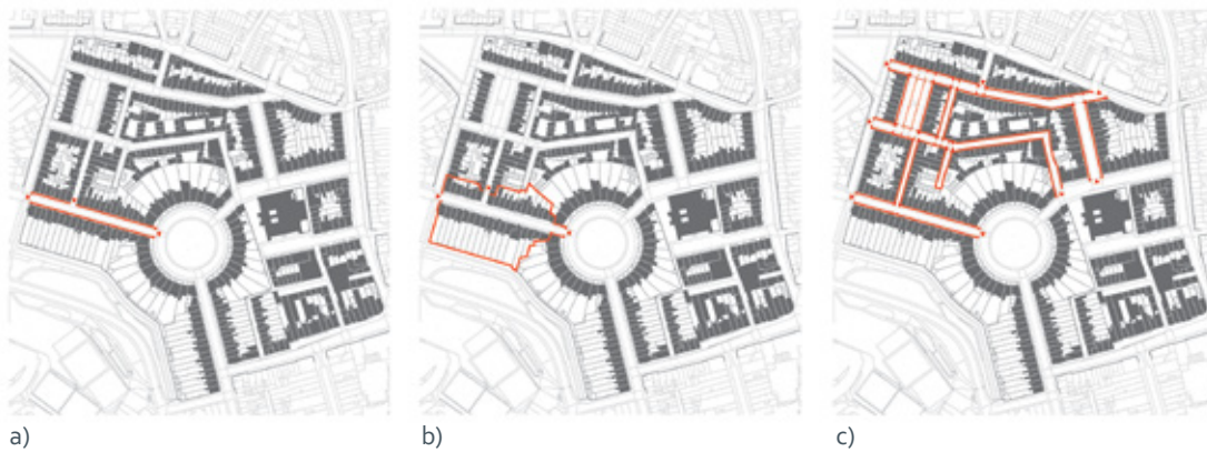
Figure 6 - a) A street space; b) the street space embedded in a simple tissue and c) an aggregate of street spaces forming a network
