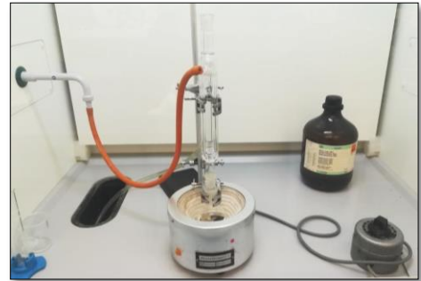
Figure 2: Sample placed in oven at 530C (left) and reinforcement left behind after burn-off (middle); Acid Digestion Set-up (right)
