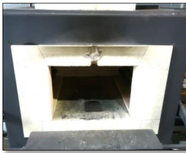
Figure 2: Sample placed in oven at 530C (left) and reinforcement left behind after burn-off (middle); Acid Digestion Set-up (right)
