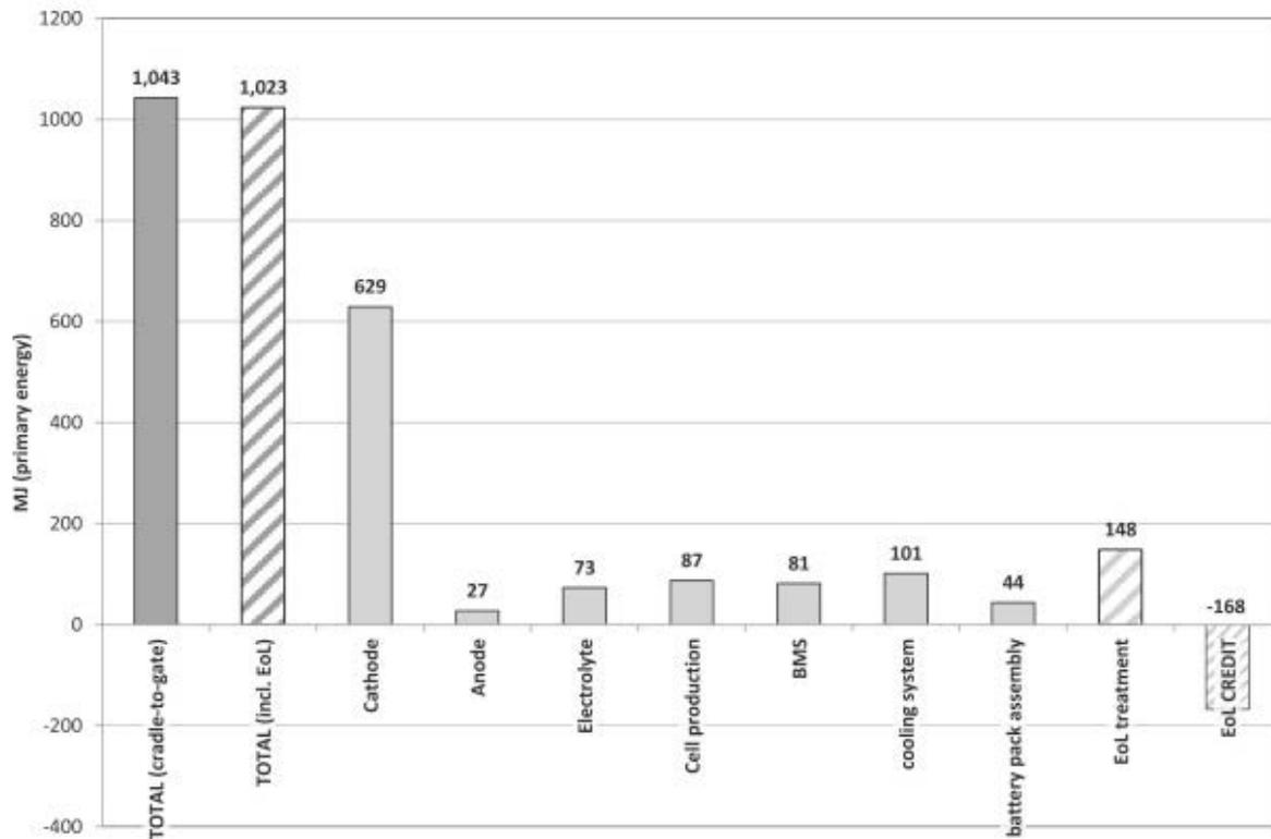
**Figure 2** – Cumulative energy demand (CED) per kWh of battery energy capacity, with and without end-of-life (EoL), and highlighting the individual contributions of the main components (BMS = battery management system).
