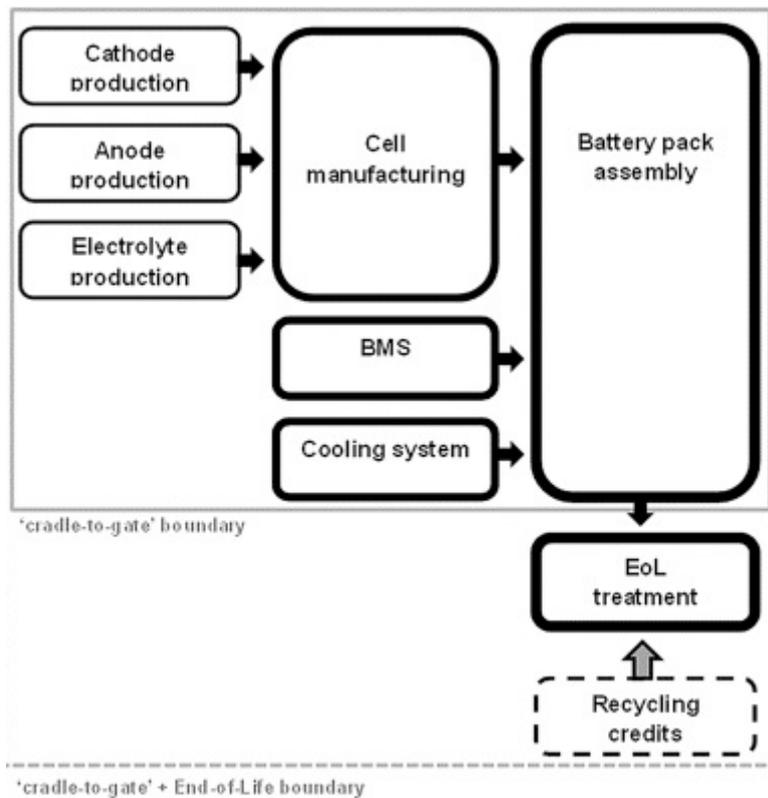
**Figure 1** – Flow diagram of the main steps in the manufacturing of a complete Li-ion battery pack, with indication of separate assessment of end-of-life (EoL) treatment and associated recycling credits.
