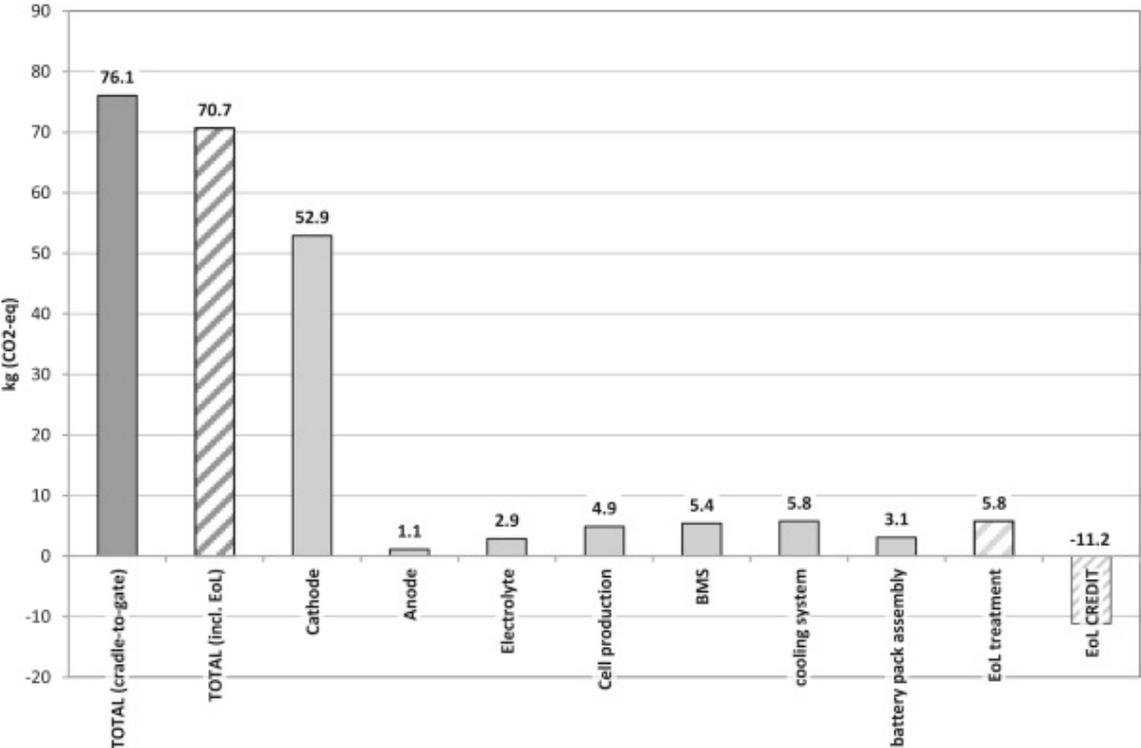
**Figure 3** – Cumulative greenhouse gas (GHG) emissions per kWh of battery energy capacity, with and without end-of-life (EoL), and highlighting the individual contributions of the main components (BMS = battery management system).
