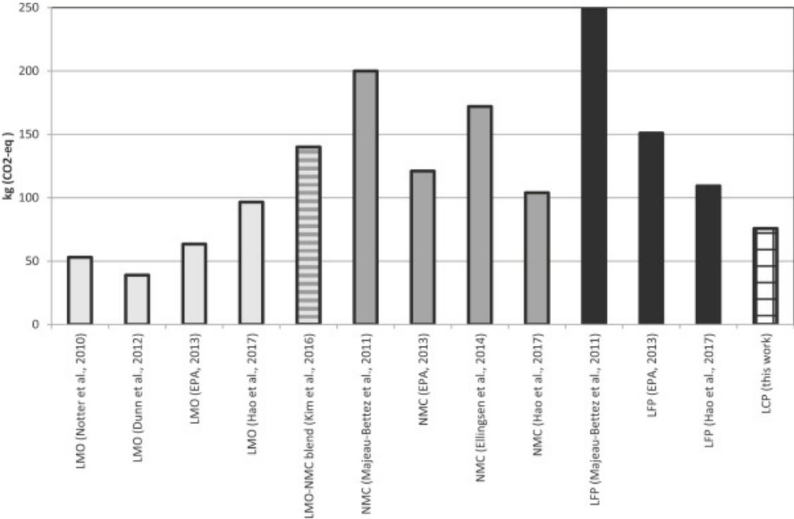
**Figure 4** – Comparison of the reported cumulative greenhouse gas (GHG) emissions per kWh of battery energy capacity across selected published studies (‘cradle-to-gate’ boundary).
