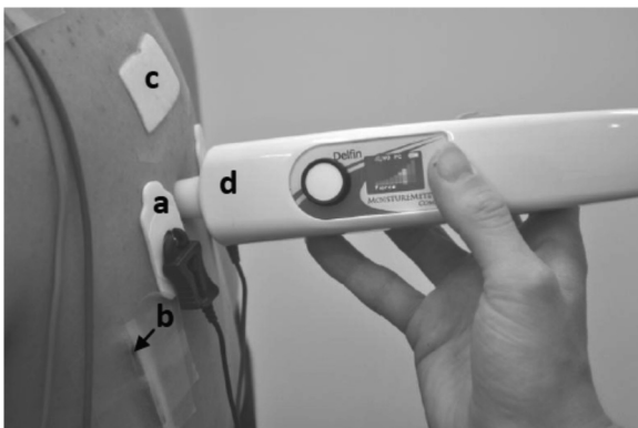
Fig. 2. The measurement area of the upper back indicating the location of an electrode for \Delta galvanic skin conductance ( \Delta\text{GSC} ; a), thermistor for skin temperature (b), absorbent patch for regional sweat rate (RSR; c), and MoistureMeterSC for epidermal hydration (HYD; d), which was applied periodically.
