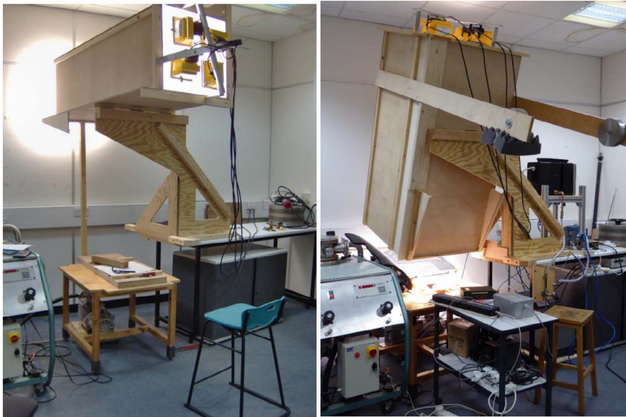
Fig. 5. (a) Simulator with light tube swung upwards for access to target area and lamps. The variable transformer is on the bench. This was prior to the addition of the counterweights. (b) Simulator in use.
