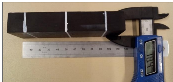
Figure 4 - Thick beam for short beam strength testing
