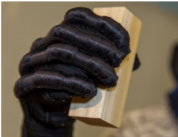
Harvard BioDesign Lab, Soft Robotic Grip Glove with fiber actuators. Photo: Harvard BioDesign Lab
