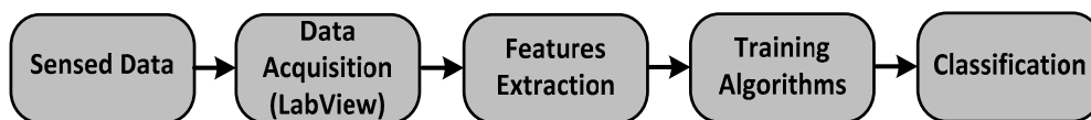
Figure 11. Overall data acquisition, feature extraction and data classification analysis flow for the gait analysis system using our WGAS.
