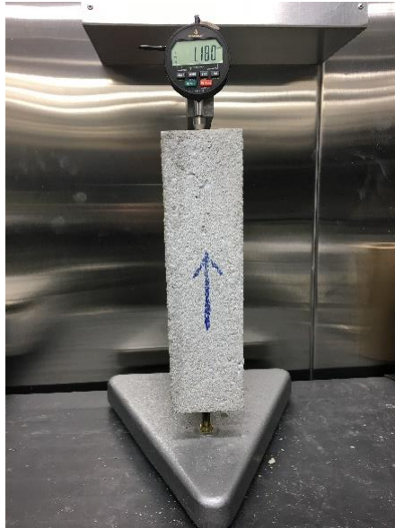
Figure 3.18. Length comparator used for shrinkage measurement
