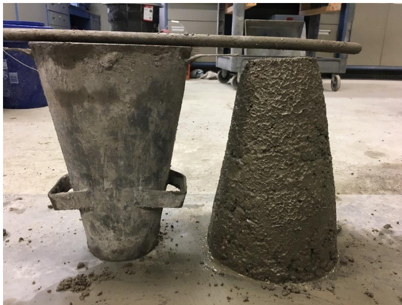
Figure 3.6. Slump test setup
