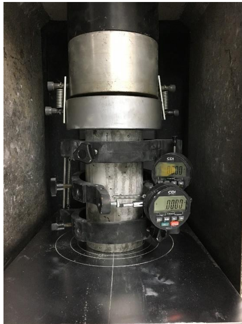
Figure 3.15. Static Modulus of Elasticity test setup
