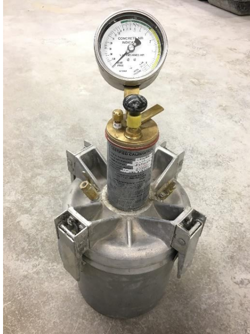
Figure 3.7. Air pressure meter
