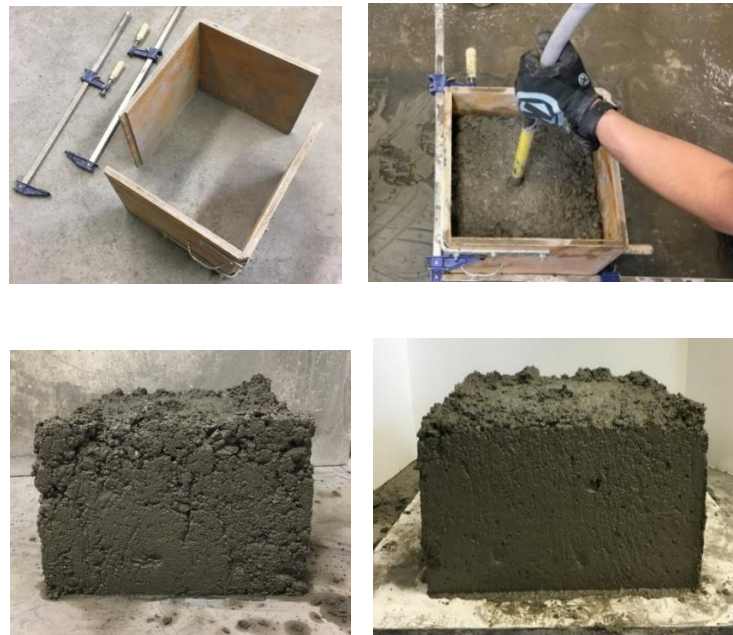
Figure 3.9. Box test setup
