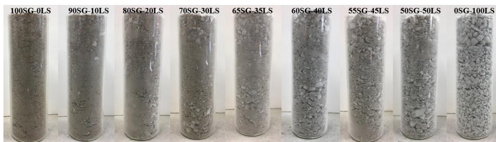
b) Visual examination of aggregate packing with different combinations
