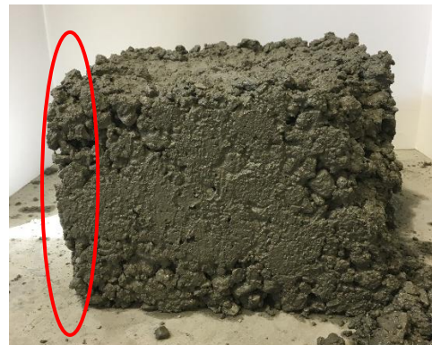
d) 4a-failed edge quality
