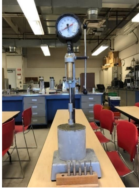
Figure 3.8. Setting time test setup
