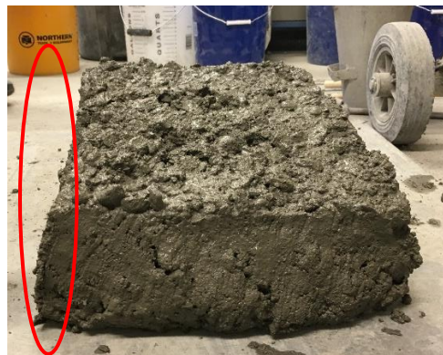
e) 4b-failed edge quality (abundance of excess paste)
