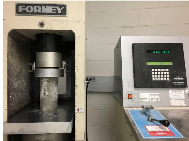
Figure 3.13. Compressive strength test setup
