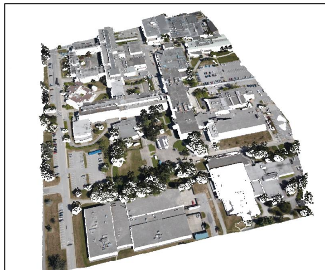
Figure 31. Realistic 3D surface reconstruction outcome for the second dataset: a single view of the textured planar surfaces and individually colored non-segmented points.
