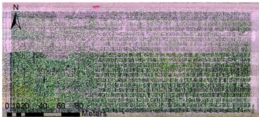
Figure 10. RGB-based orthophoto of the test field derived from the captured frame images on 25 July 2015.
