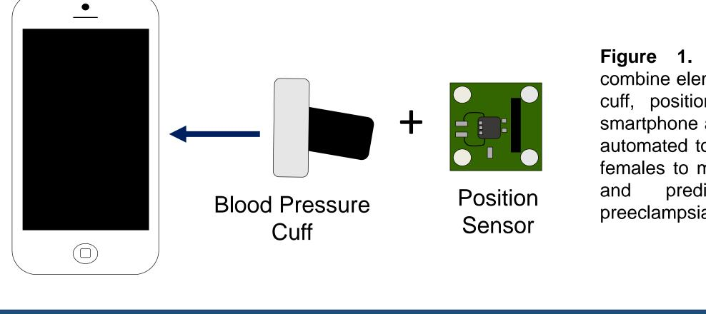
Figure 1. We want to combine elements of the BP cuff, position sensor, and smartphone app to make an automated tool for pregnant females to monitor their BP and predict risk of preeclampsia
