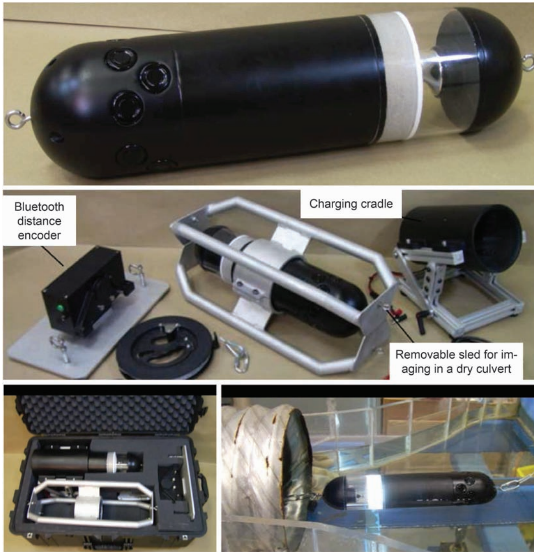
Figure 5.12 The UCIS device, parts, case in laboratory testing. Jointly developed by SwRI and FHWA.
