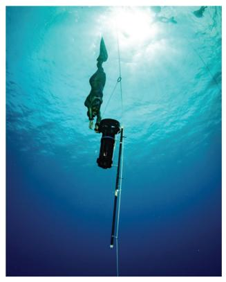
Figure 3. A freediver utilizing a DPV to aid in the descent. [Photo credit: Eiko Jones]
