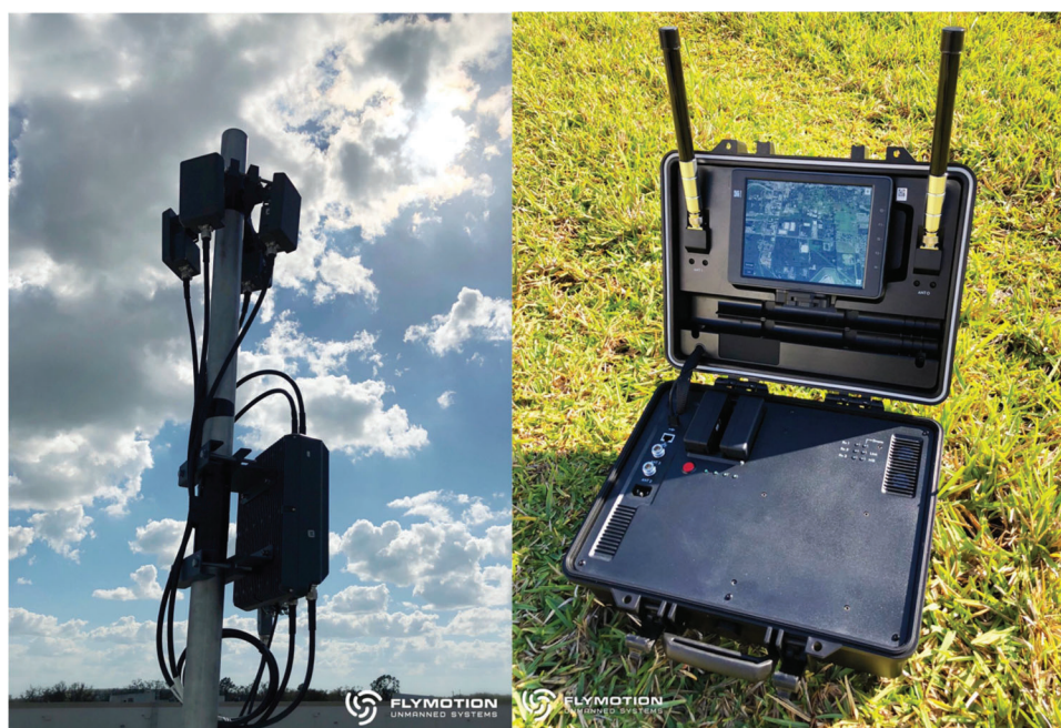
Figure 1. (Left) Permanent AeroScope radiofrequency detection device. (Right) Mobile AeroScope in Pelican case. Images courtesy of FLYMOTION. Used with permission.
