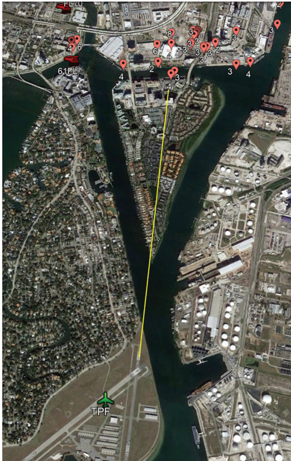
Figure 13. Visual approach path to Peter O. Knight (TPF) Runway 18. Yellow line extends from threshold (Runway 18 has a displaced threshold) along runway orientation to 1.4 SM. At the northern end of the yellow line, an aircraft performing a standard 3^\circ approach would be at approximately 387 ft AGL, based on trigonometric calculations. Assuming detected activity is representative of normal UAS flight operations north of Harbour Island, this condition would likely put approaching aircraft coming into Runway 18 at a risk of midair collision.
