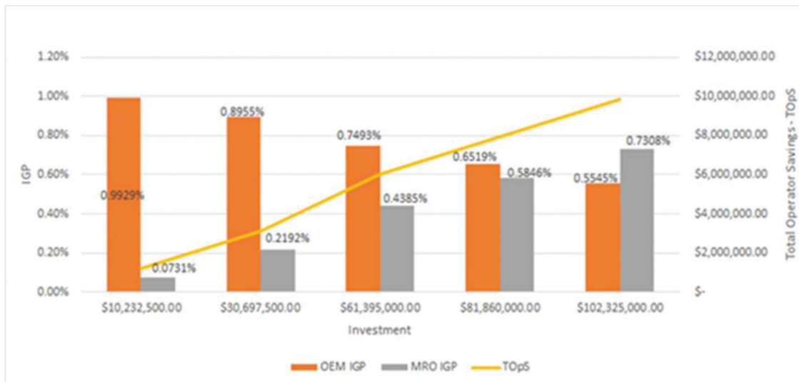
Figure 6. PSS2 impact on GP versus total operator savings (80% investment from OEM and 20% investment from MRO firm).
