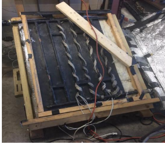
Figure 2(b) Collector for the indoor thermosiphon test facility
