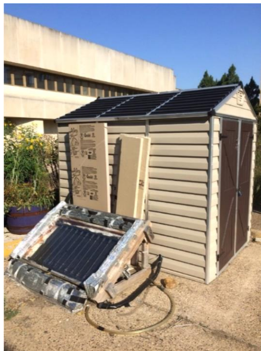
Figure 3 Solar collector with glazing connected to a heat exchanger contained in the outdoor facility
