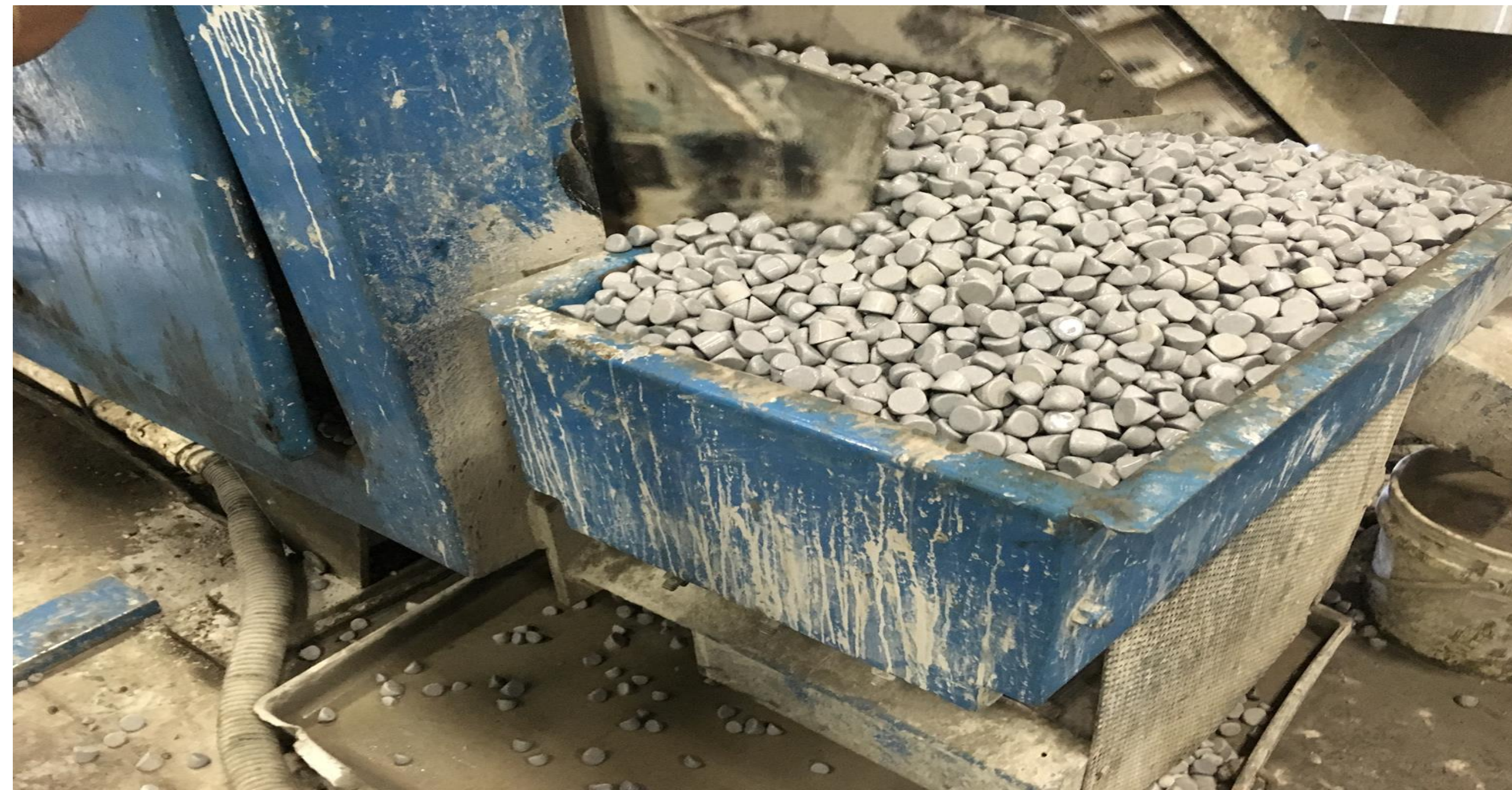
Fig. 1. A view of media falling out of the hopper as the system runs.
