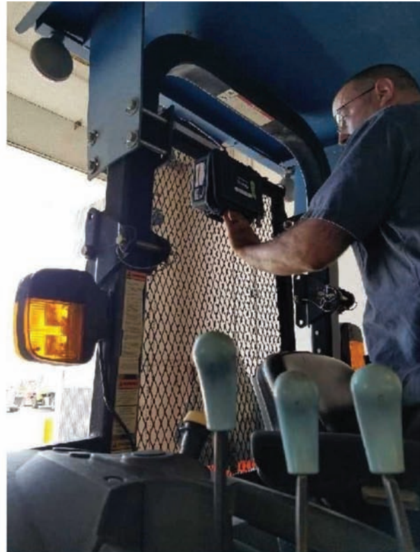
(b) Installation of GPS device on the mesh behind driver seat
