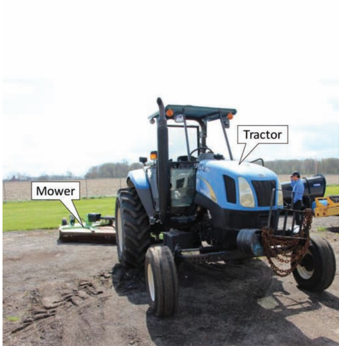
(a) Tractor with 15' flex-wing rotary mower
