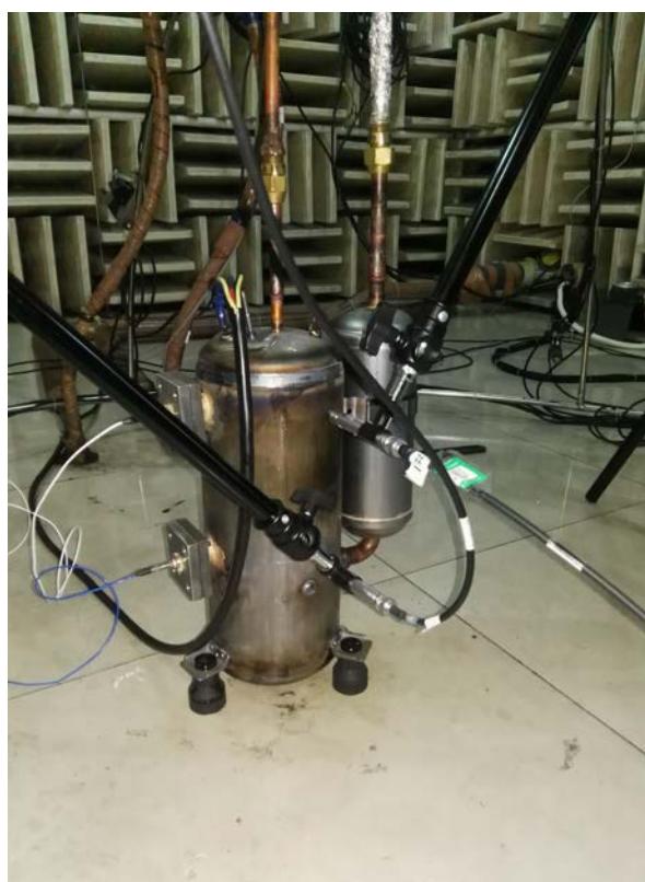
Figure 1: Pressure pulsation test fixture of rotary compressor
