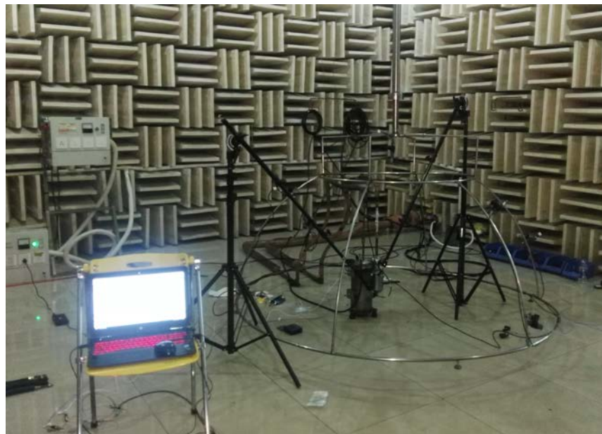
Figure 7: Noise test fixture
