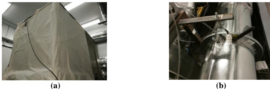
Figure 3: (a) Light Condenser fouling simulated by a layer of fabric placed on the condenser surface (b) Iris damper used for simulating evaporator fouling equipped with a black screw for adjusting its opening.
