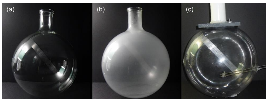
Figure 2: Color images of the vessels used. Shown here are: (a) a new glass vessel; (b) a glass vessel that has been etched by 10 flame tests followed by immediate flushing; and (c) a polycarbonate vessel following 68 similar tests. Behind each vessel is a 30 cm ruler.
