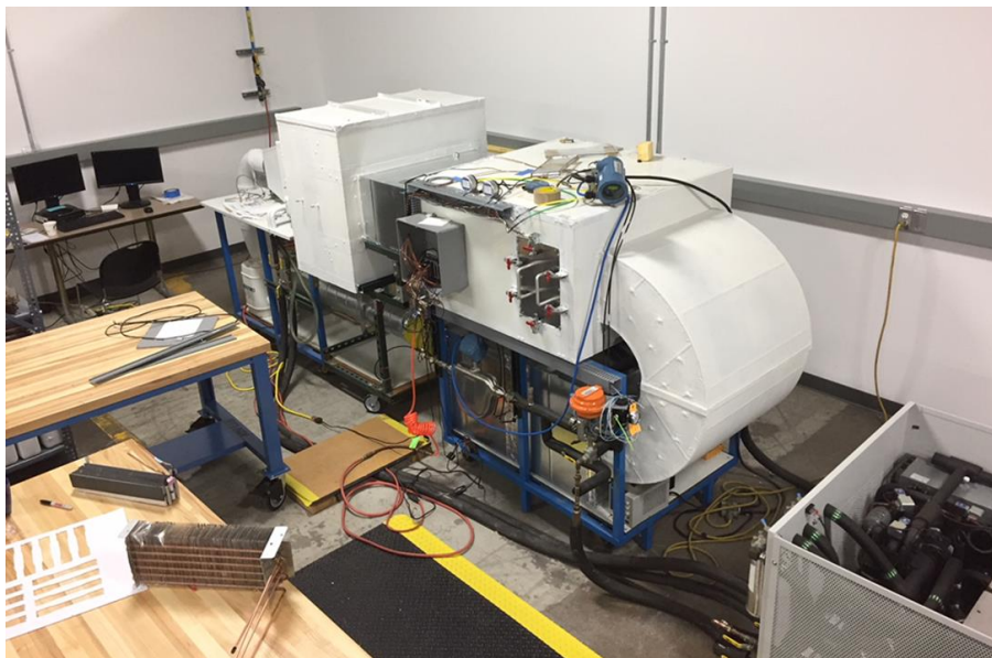
Figure 6: Hot water calorimeter
