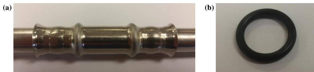
Figure 2: (a) 1/2" stainless steel press/crimp fitting and (b) 1/2" HNBR O-ring.
