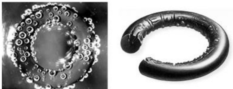
Figure 3: Images of O-ring failures due to explosive decompression (left image from Seal & Design, right image from Marco Rubber & Plastics).
