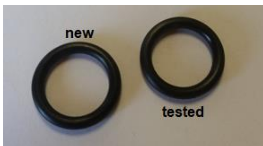
Figure 7: Visual comparison of decompression tested (dry) and new/untested O-rings shows no detectable damage to the O-ring that underwent 10 rapid decompression tests.
