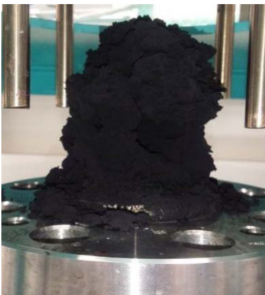
Fig. 8. Soot production during the disproportionation reaction.
