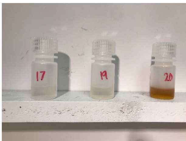
Figure 9: Exposed Oil Samples using HFO-1234yf (left to right: 17, 19, and 20)
