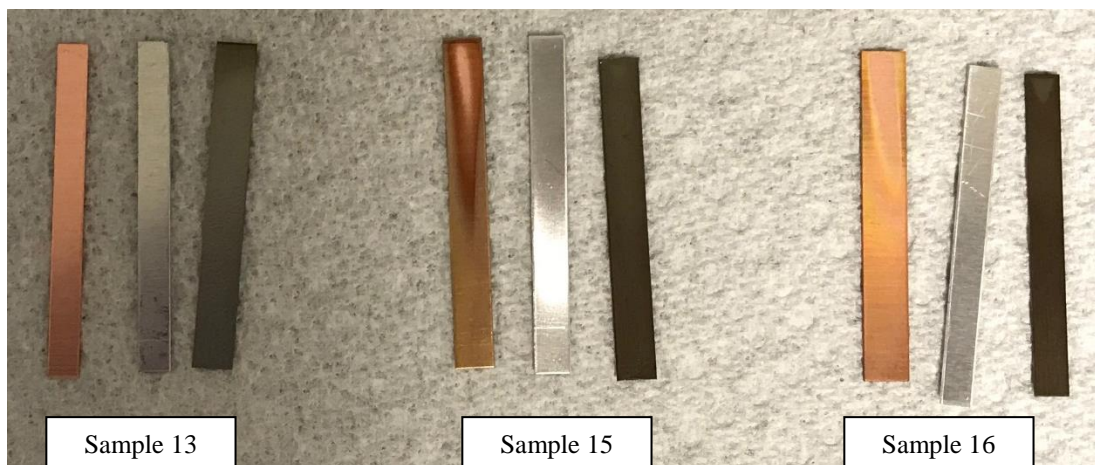
Figure 10: Exposed Metal Coupons using HFC-134a
