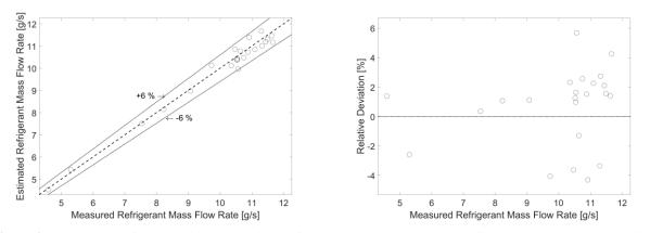
Figure 2: Parity plot (left) and residual plot (right) of compressor training set mass flow rate measured vs. predicted values
