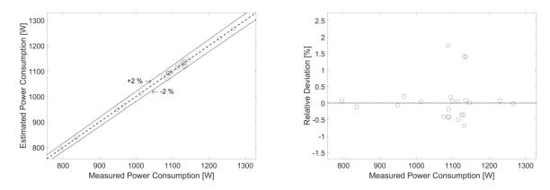
Figure 6: Parity plot (left) and residual plot (right) of compressor training set power consumption measured vs. predicted values
