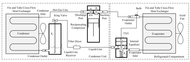
Figure 1: Schematic diagram of a walk-in refrigeration system
