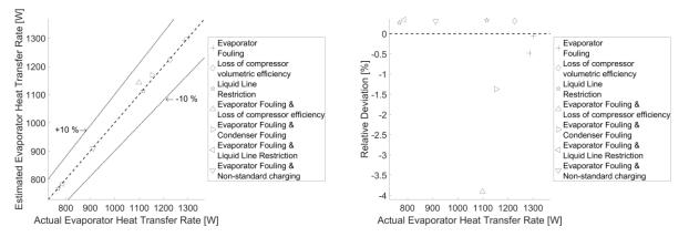
Figure 5: Parity plot (left) and residual plot (right) of evaporator validation set heat transfer rate actual vs. predicted values
