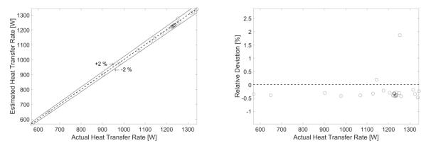
Figure 4: Parity plot (left) and residual plot (right) of evaporator training set heat transfer rate actual vs. predicted values
