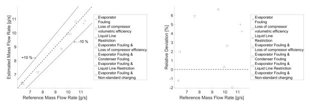
Figure 3: Parity plot (left) and residual plot (right) of compressor validation set mass flow rate measured vs. predicted values
