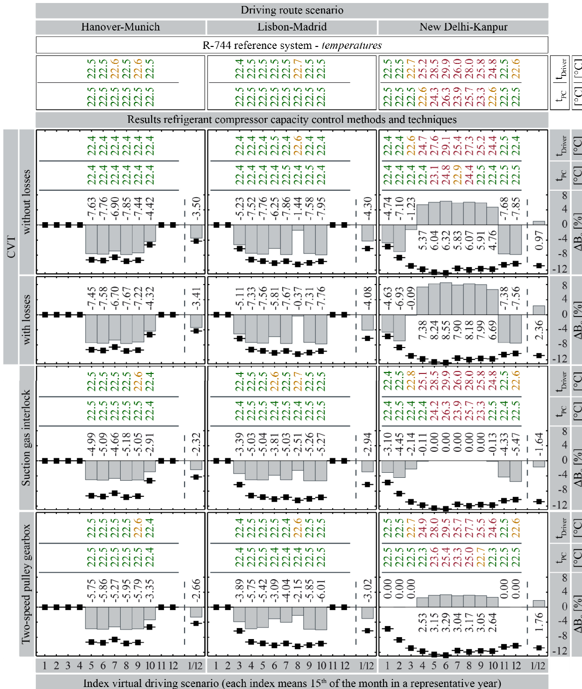
Figure 7: Numerical results of individual application of the ideal and more realistic CVT as well as of the suction gas interlock and the two-speed pulley gearbox for an R-744-based air conditioning system. Shows the fuel consumption of each monthly driving scenario and, in the last column of each diagram, the average annual fuel consumption (1/12). Black boxes present the theoretical limit potential of fuel savings through operation of the air conditioning system.
