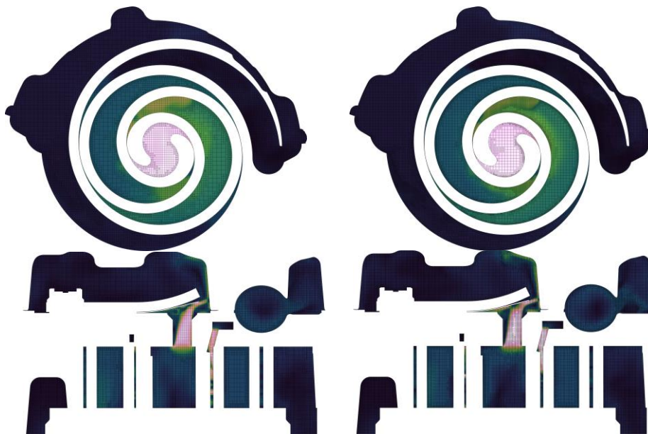
Figure 11: Planes colored by temperature (top) and velocity (bottom) for two grids in the convergence study. The left is Grid-3, and to the right is Grid-4 as described by Table 2.
