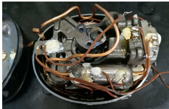
Figure 3: The distribution of the thermocouples inside the shell
