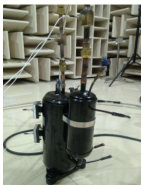
Figure 2 (a) :Photos of compressor pressure pulsation testing
