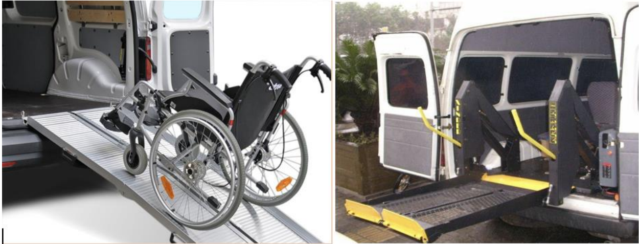
Figure 10: A ramp and lift; respectively, are two of the most common mechanisms used by travelers using wheelchairs to board a vehicle.
