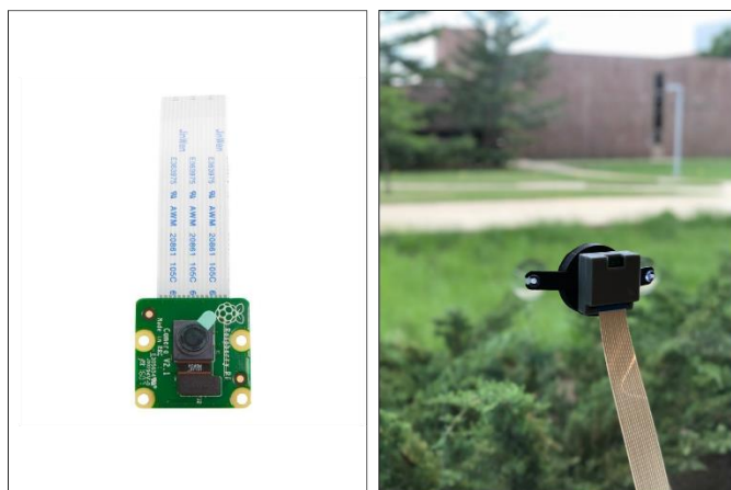
Figure 1: Camera-on-board chipset (left) – Finalized window sensor with 3D-printed case and mount (right)
