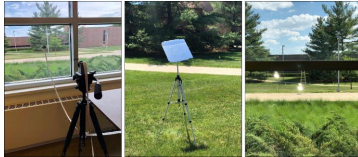
Figure 10: Dual camera setup (left), Reflector mount (center) – Reflectors as seen from the observer position (right)
