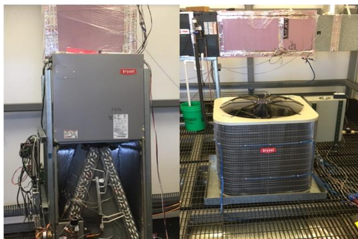
Figure 3. Variable-speed split heat pump setup for frequency regulation testing
