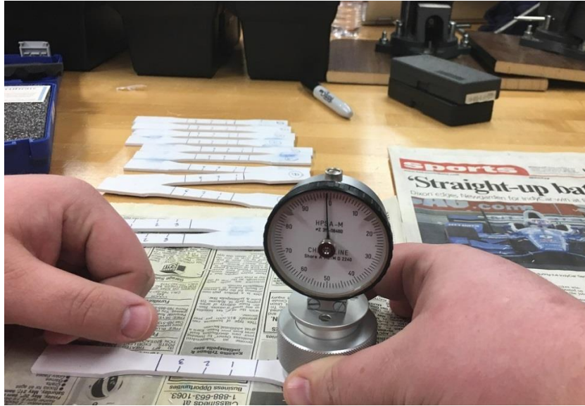
Figure 4 Shore Durometer is used to measure the hardness of a PS specimen
