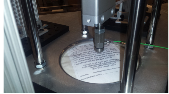
(b) Impactor Controlled by Actuator
