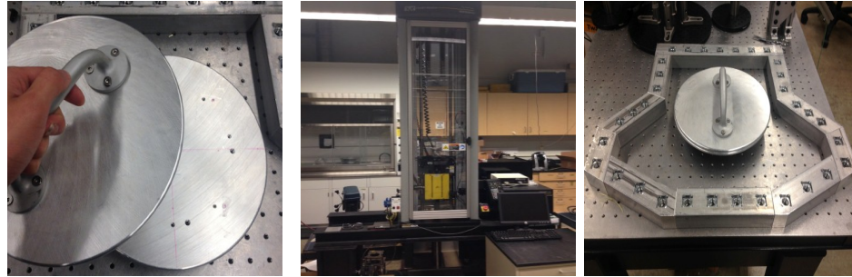
(a) Upper and Base flat- (b) Drop tower mechanism (c) Base fixture for the tender alignment of the frames
