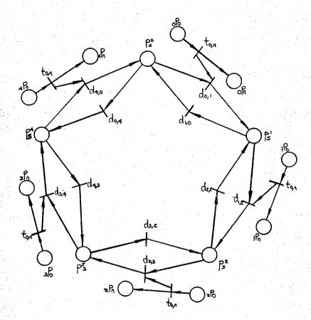
Figure 3. Petri-net representation of a distributed computation with five nodes and two phases.
