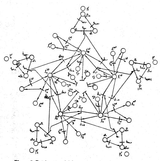
Figure 5. Petri net model for a distributed computation with 5 computation nodes and 3 phases associated with each node.
