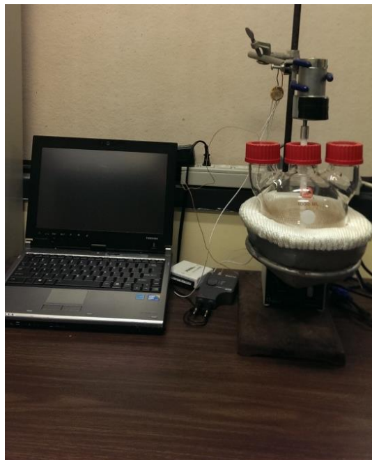
Figure 3.38 Picture of the in-house built universal sensor gas characterization system (Panigrahi et al., 2008)
